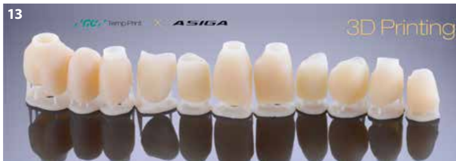
Fig. 13: Second set of provisional restorations printed with GC Temp PRINT (medium shade) using the Asiga Max UV 3D printer.
