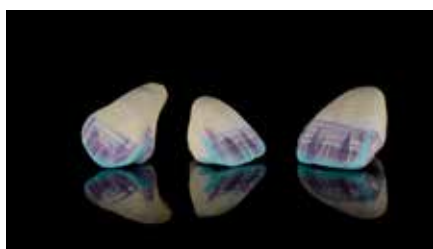
Fig. 5: Zirconia crowns coloured with Initial Zirconia Coloring Liquid before sintering.
